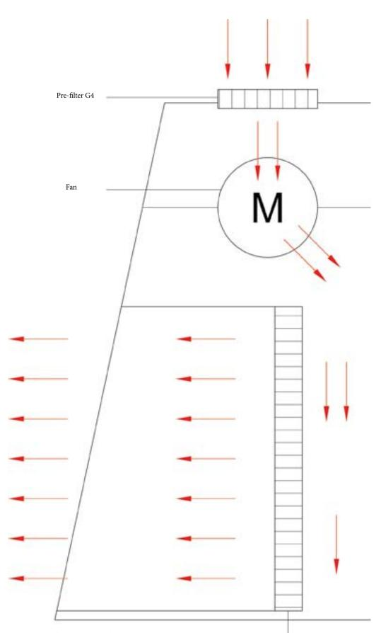
The cross-section above shows the working of the cross flow unit
